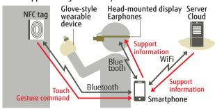
occurs. This extends the operational time for a glove-style wearable device from 3 hours in the absence of electric power control to 9 hours, achieving operating time sufficient for a day's work.
