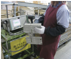
Plastic material identification equipment
