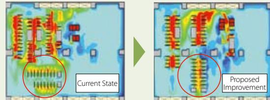
Air Flow and Temperature Distribution Simulation Example (floor plan)
