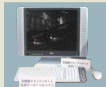
A prototype PC using plastic with a photocatalyst additive
