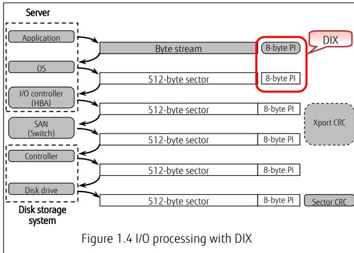
Figure 1.4 I/O processing with DIX
