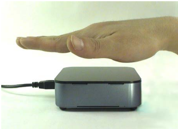
Contactless palm vein recognition unit
