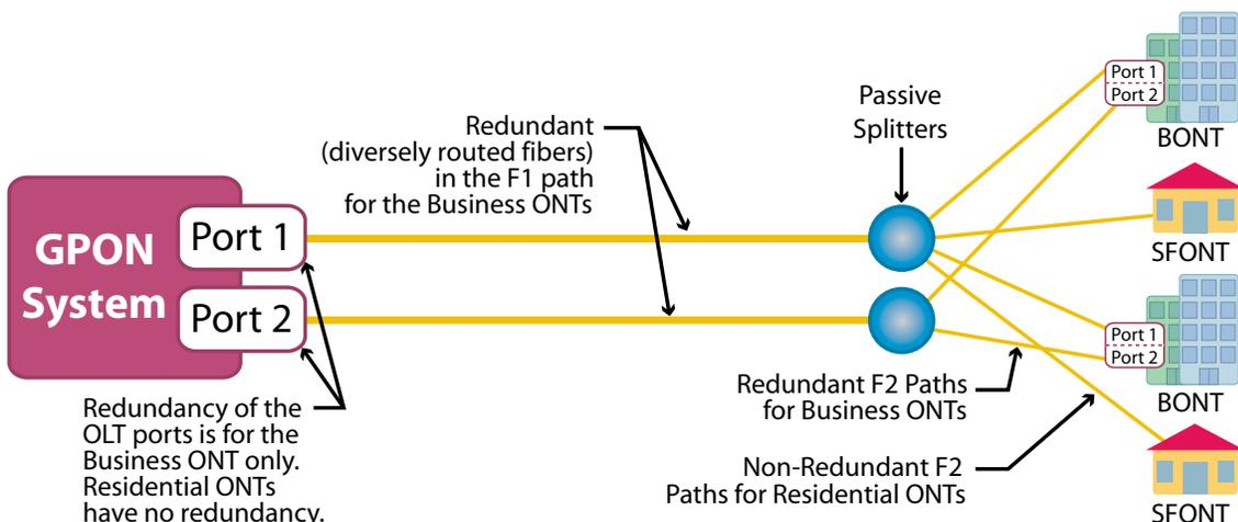
**Figure 5: Type C Redundancy Scheme**
