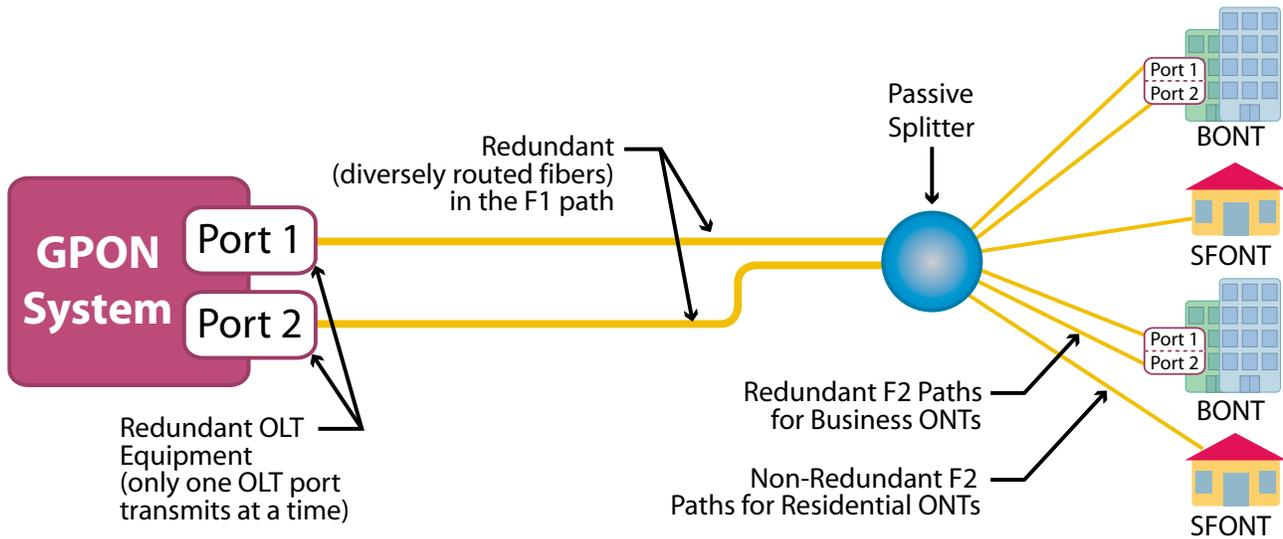
**Figure 4: Type B Protection Scheme**
