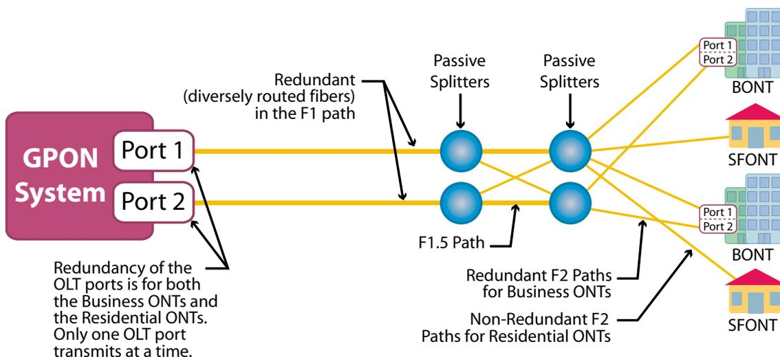
**Figure 6: Type D Redundancy Scheme**
