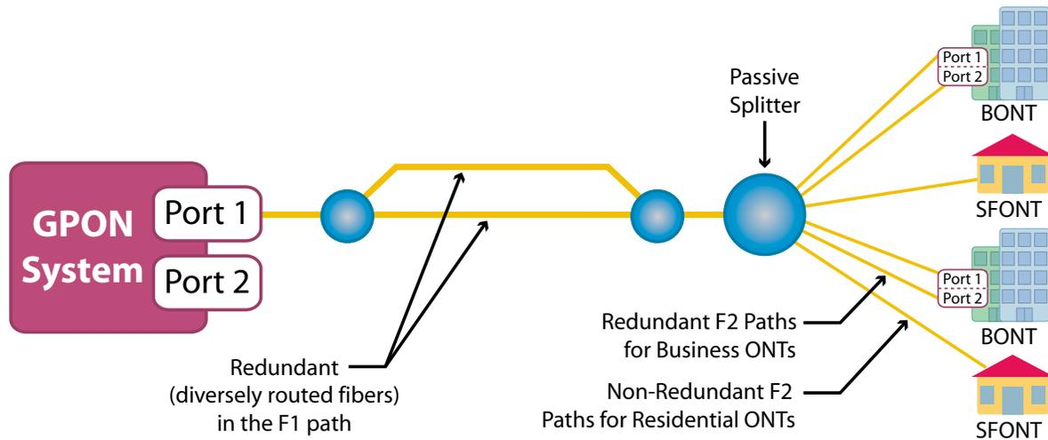
**Figure 3: Type A Protection Scheme**
