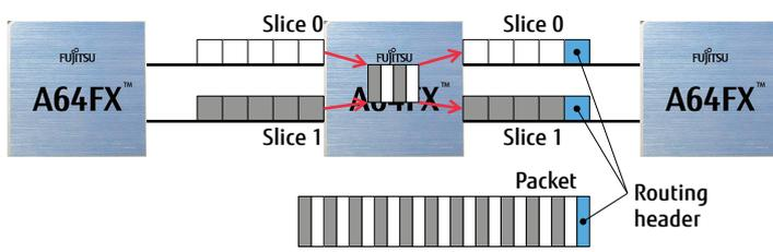
Figure 15 Dynamic packet slicing: Split mode
