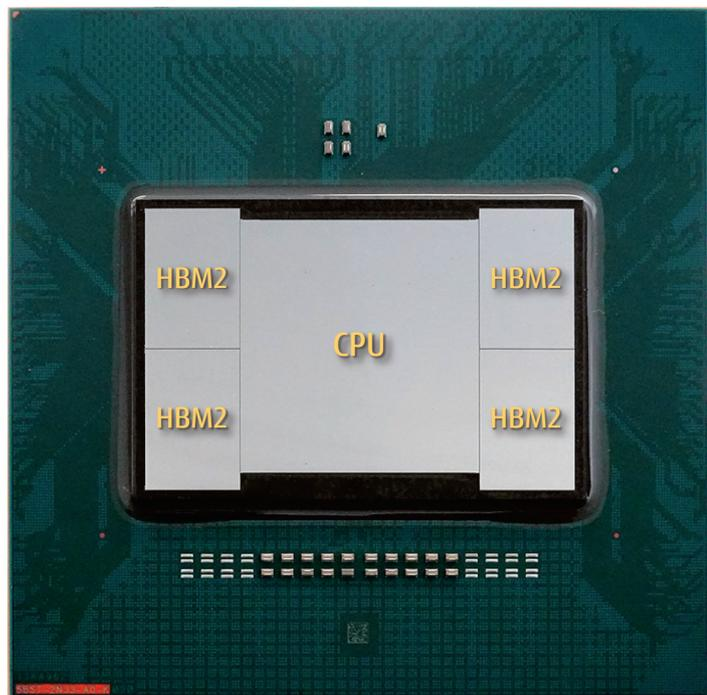
Figure 11 Photograph of the A64FX 2.5D package
