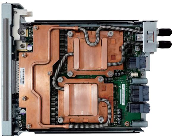
Figure 1 PRIMEHPC FX1000 CPU memory unit
