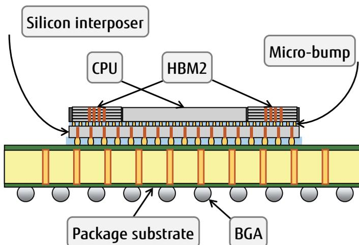
Figure 12 2.5D package structure (schematic sectional diagram)
