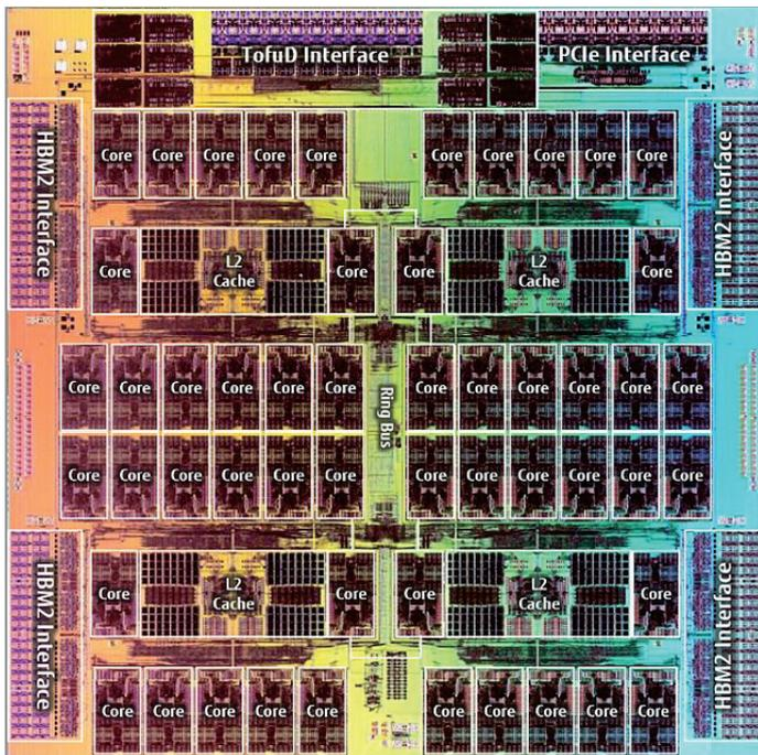
Figure 3 Photograph of the A64FX CPU chip
