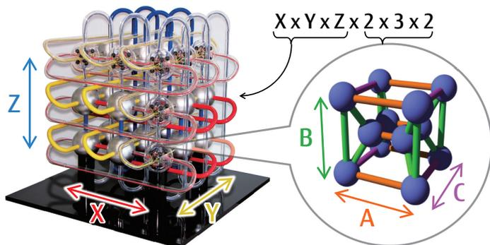
Figure 13 6D mesh/torus topology model
