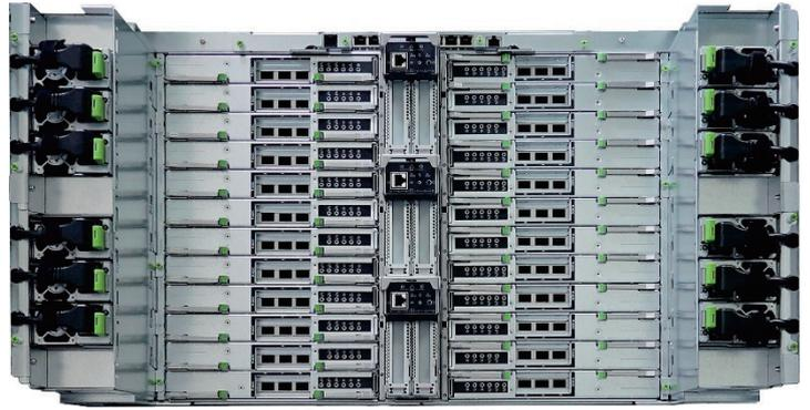
Figure 2 PRIMEHPC FX1000 main unit
