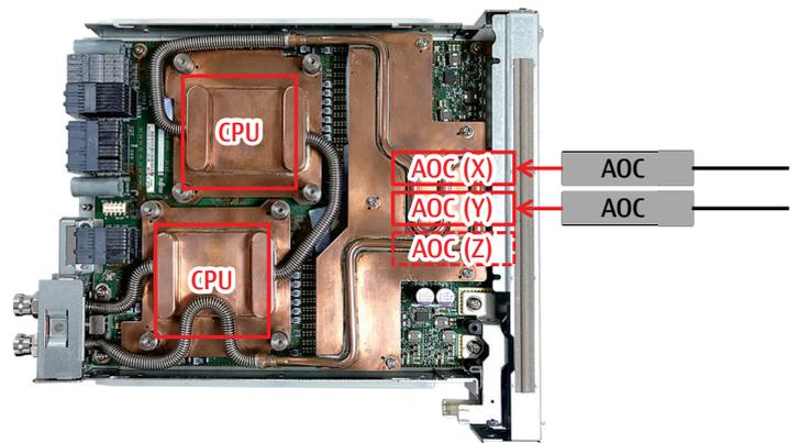
Figure 14 AOC connections to a CMU
