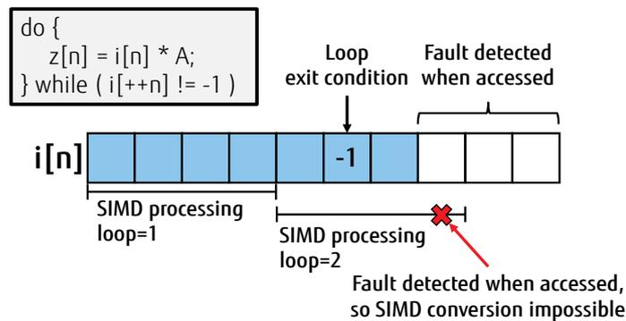
Figure 8 Difficulty of converting a Do-while loop into SIMD
