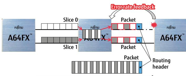
Figure 16 Dynamic packet slicing: Duplicate mode
