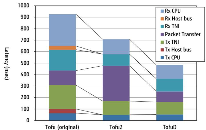
Figure 17 Breakdown of communication latency
