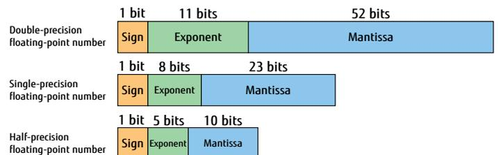
Figure 6 Supported floating-point number formats
