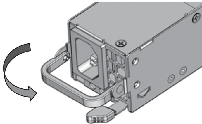
2. Push in the PSU (1) until the latch clicks and locks in place. Fold back the handle on the PSU (2).
