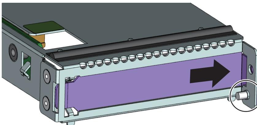
2. Pull the slot cover out of the riser module in the direction of the arrow.
