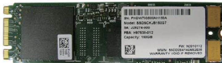
1. With the M.2 SSD slightly tilted and the label facing up, insert the M.2 SSD into the M.2 slot.
