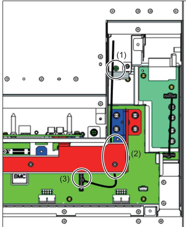
3. Pass the cable under the bus bar (2).
