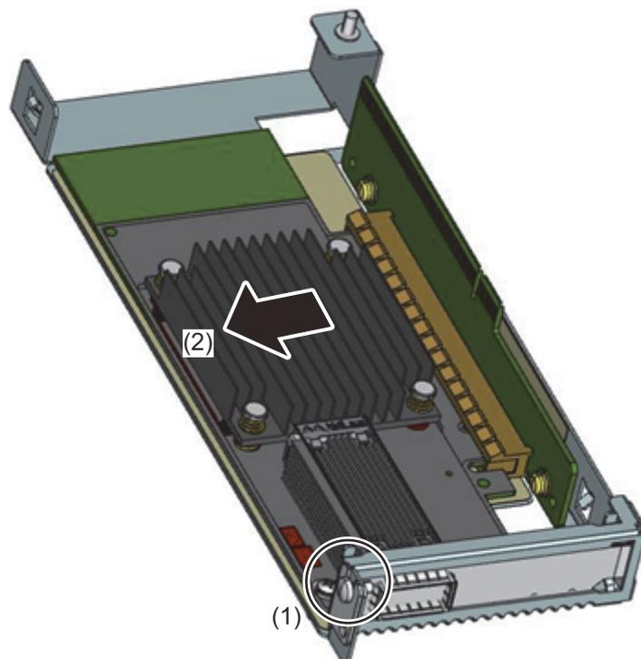
2. Pull out the InfiniBand card from the riser card connector (2).
