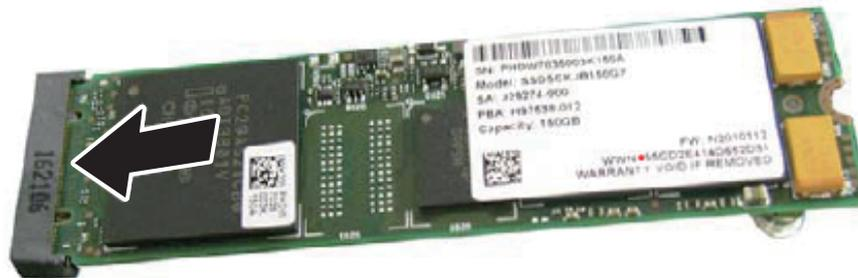
2. Secure the M.2 SSD to the standoff spacer with one screw.
