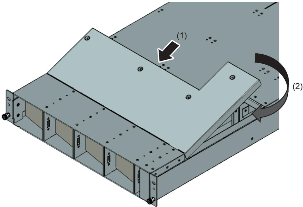
2. Secure the top cover with screws.
