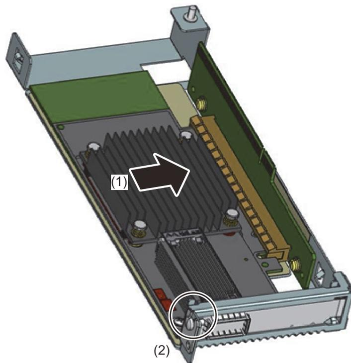
3. Secure the InfiniBand card with one screw (2).
