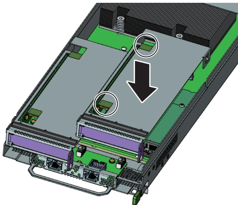
2. Secure it with a fixing screw. (Circled part)
