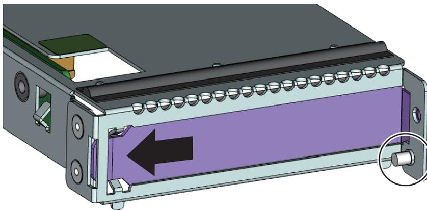
2. Secure the slot cover to the riser module with a screw. (Circled part)
