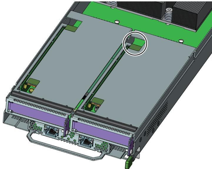
3. Lift and remove the riser module.
