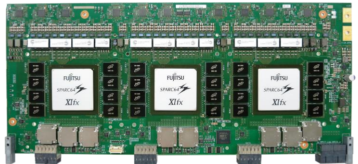
Figure 11 High-density packaging of CMB
