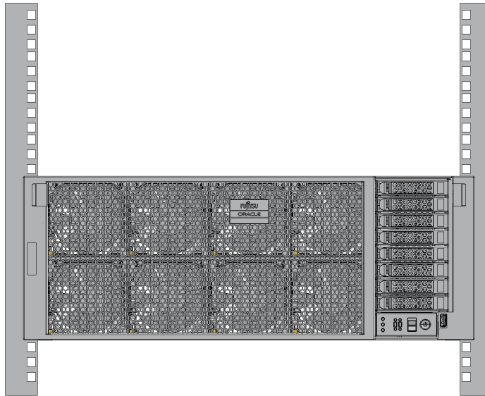
Figure 3-45 SPARC M12-2S Mounting Completed (Front)
