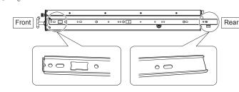
6 Attach the left rear holding bracket (CA32476-Y766) to the inner slide
