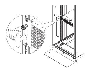
9 Release the locking lever on the inner slide rails and insert the server into the rack.
