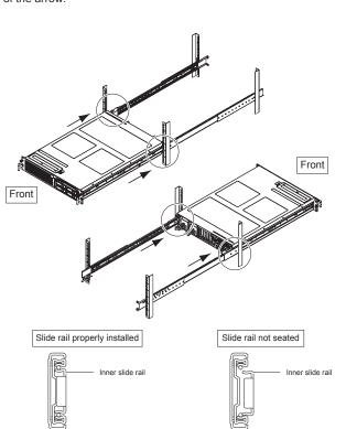
Note - With the server extended fully out on the rails and firmly supported by two people, gently shake it to make sure the server does not come off from the slide rails.
