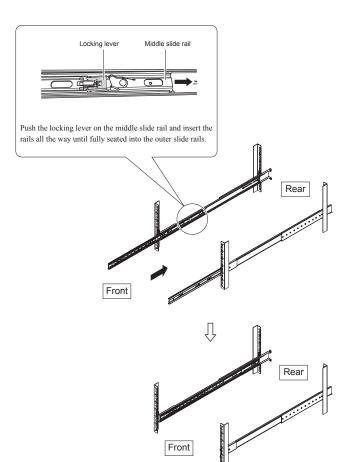
Make sure that the bearing board (thin metal sheet with oval holes) that is housed in the rails is at the front end of the rail.
