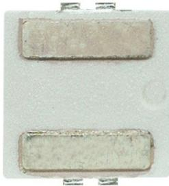
*Soldering surfaces are located on the bottom of the components.*
