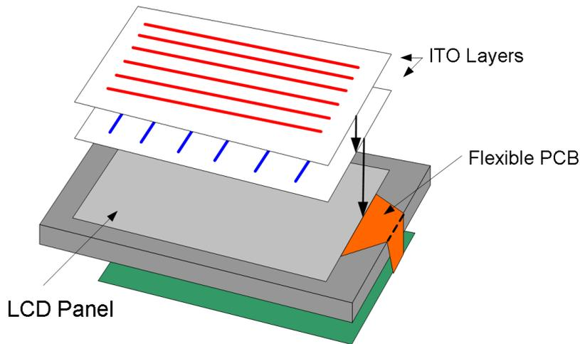
*figure 7 Capacitive touch screen with matrix arrangement*
