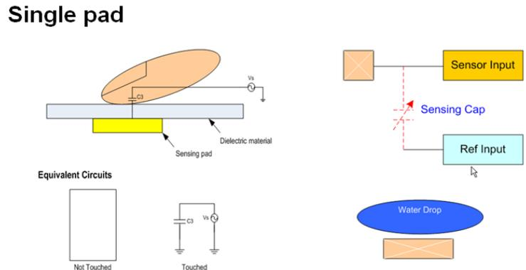
figure 6 Single sensing pad
