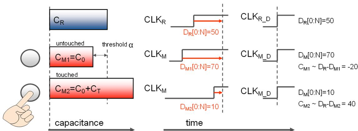
figure 3 Timing diagram of RC-delay line capacitance measurement method
