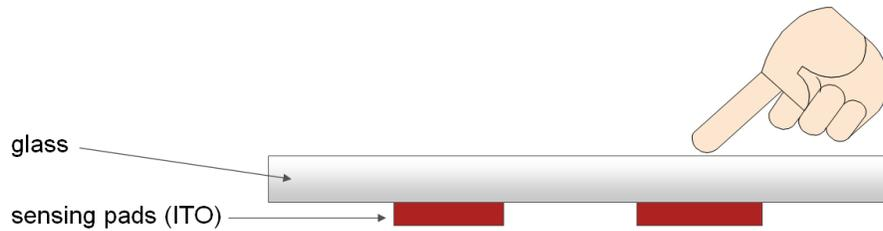
figure 8 Capacitive touch screen with discrete sensing pads, consisting of one ITO layer
