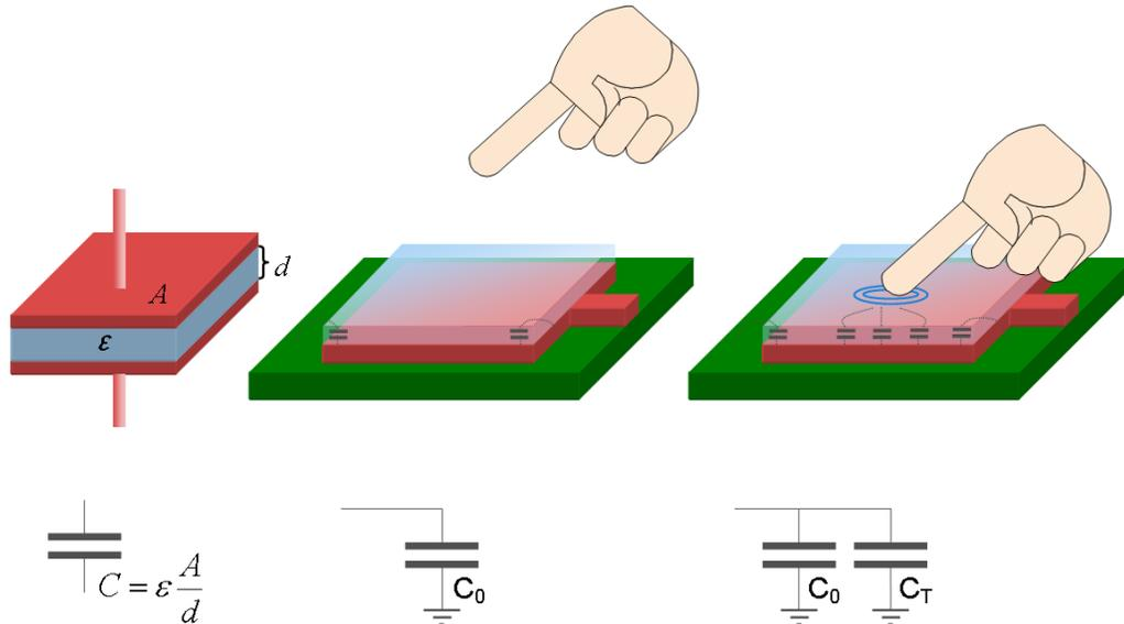
figure 1 Touch Sensor Principle: untouched sensor pad with parasitic capacitance  $C_0$ , touched sensor pad with additional touch capacitance  $C_T$ .
