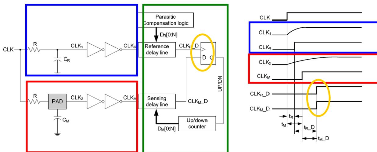
figure 2 Block diagram of RC-delay line capacitance measurement method
