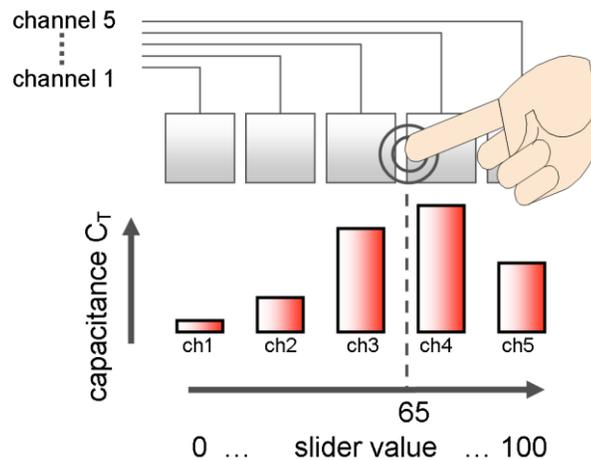
figure 4 Capacitive touch slider implementation with interpolation
