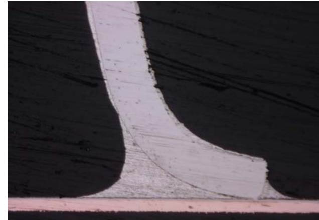
A) Paste : Eutectic Solder Lead Frame : 42-Alloy Reflow Temperature :230°C
