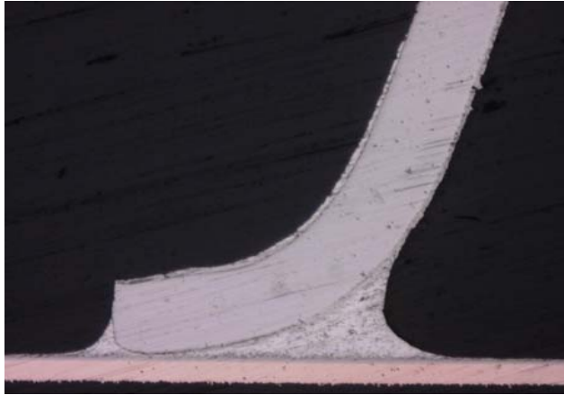
A) Paste : Eutectic Solder Lead Frame : 42-Alloy Reflow Temperature :230°C
