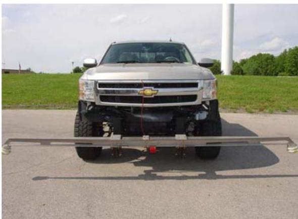
*Figure 5. Modified vehicle with custom outrigger*
