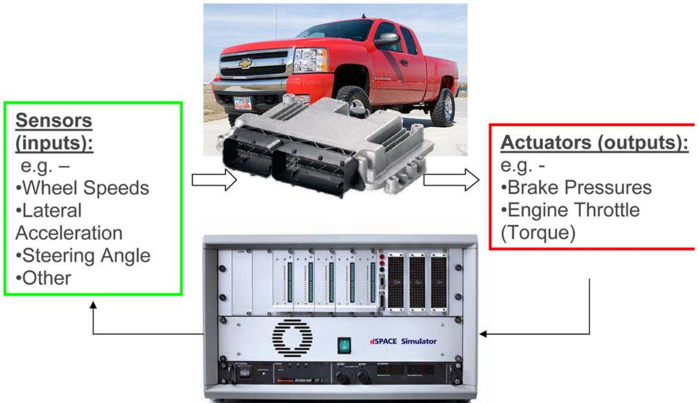
*Figure 9. Simple diagram of HIL components*
