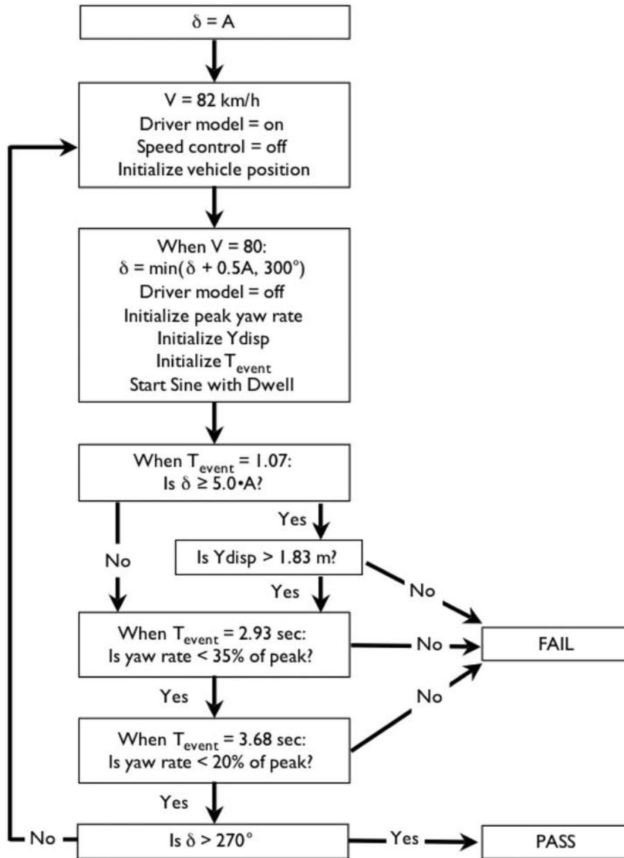
Figure 3. Flow chart for the Simulated Sine with Dwell test series
