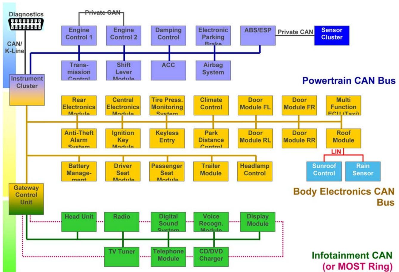
Figure 10. The Brains: Networked Electronic Control Units
