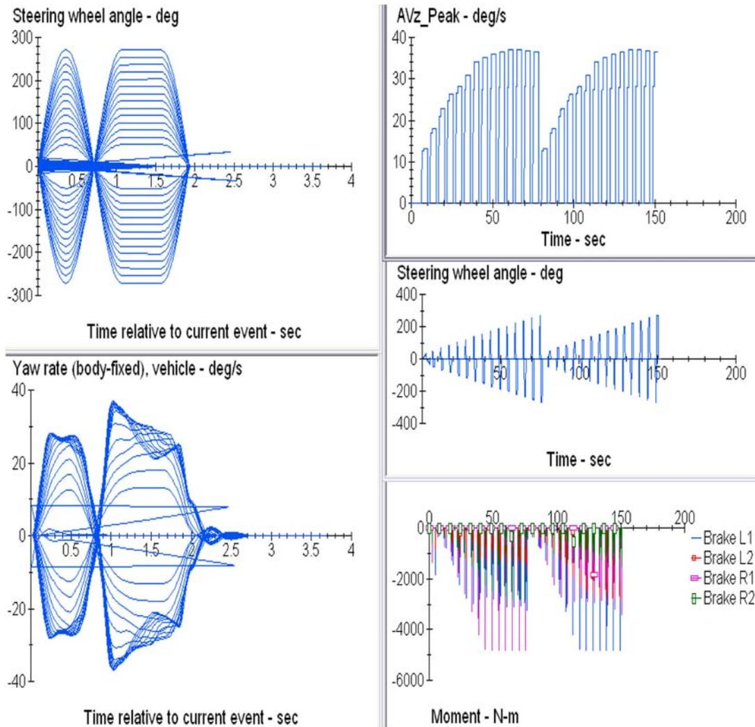
**Figure 8. Response of the vehicle with ESC for the full test sequence**
