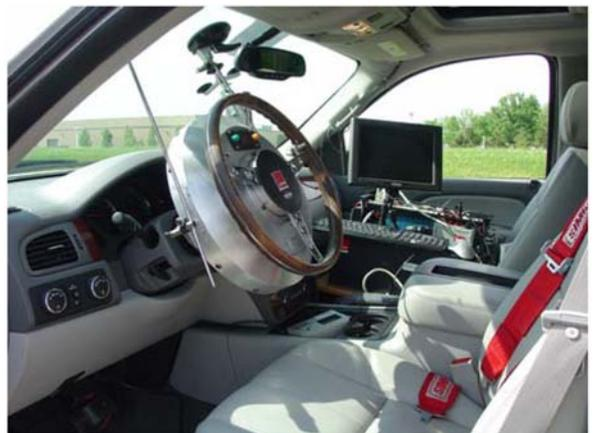
*Figure 6. Steering "robot" with instrumentation*
