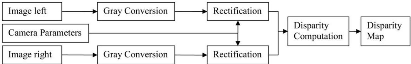
**Figure 1. Stereo system overview:** Raw images are converted to gray scale and rectified using intrinsic as well as extrinsic camera parameters. Rectified images are provided to the disparity computation module to facilitate correspondence search. The output is a disparity map containing depth information for each pixel.
