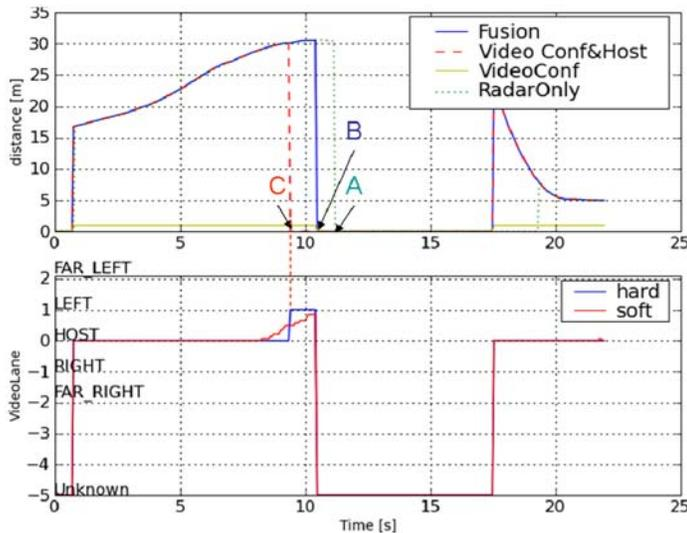
**Figure 4. ACC target release for different fusion levels.**
