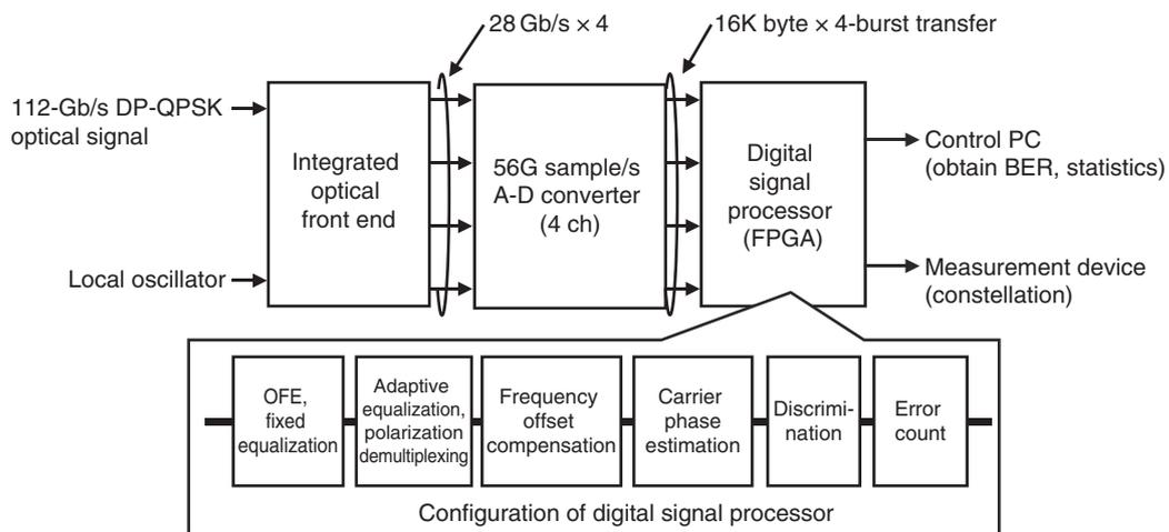
(a) Configuration of coherent receiver and signal processor
