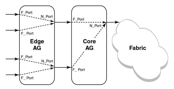
AG cascading provides higher over-subscription because it allows you to consolidate the number of ports going to the main fabric. There is no license requirement to use this feature.
