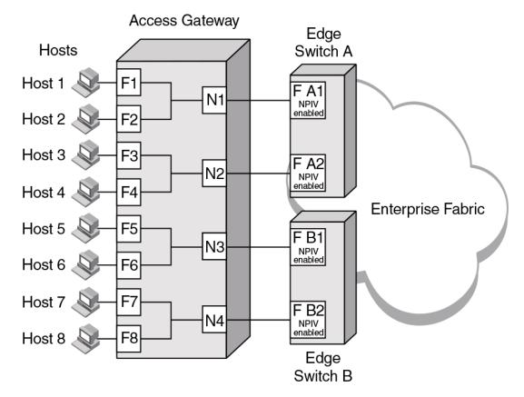
FIGURE 5 Port mapping example
