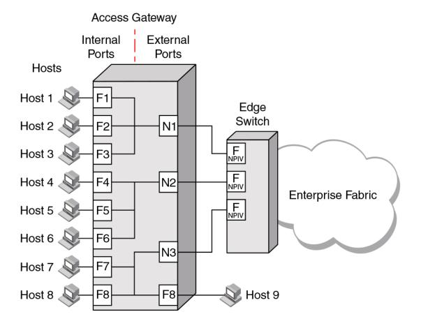
FIGURE 2 Switch function in Access Gateway mode
