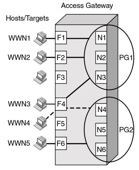
FIGURE 6 Example of device mapping to N\_Port groups
