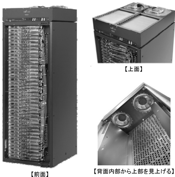
図-3 CX1000外観と集中冷却大型ファン Fig.3-Appearance of CX1000 and its large central cooling fans.
