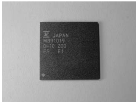
図-5 権利保護LSI Fig.5-Digital Content Rights Protection LSI.
