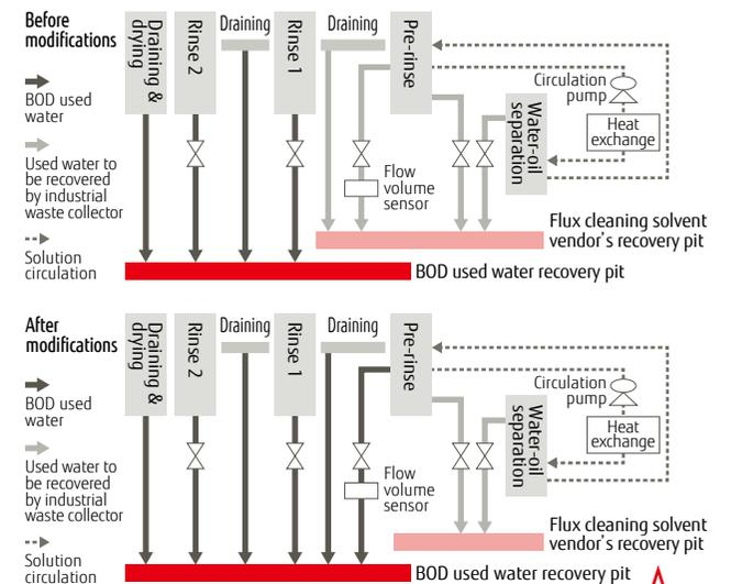
The in-house treatment system takes wastewater that has been drained or has passed through the flow sensor and re-routes it to a BOD used water recovery pit instead of the cleaning solvent vendor's recovery pit.
