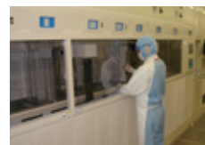
Adjusting pure water flow to manufacturing machinery
