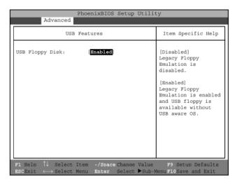
Figure 11. USB Features Submenu
