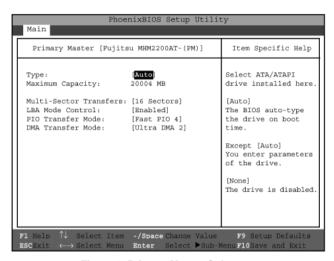
Figure 2. Primary Master Submenu
