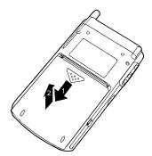
• Slide the Full Reset switch to the right with the stylus.
