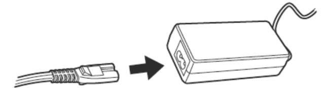
2. Insert the connectors of the AC adapter into the scanner power inlet and a power outlet.
