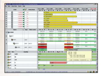
Factory Planning enables the seamless execution of the production plan by having shop floor terminals interrogate the application for the correct and current work queue at each work center. The operators simply select the correct item from the list, which "starts" the operation. You can also call up data, drawings, work instructions and additional information from the remote terminal.
