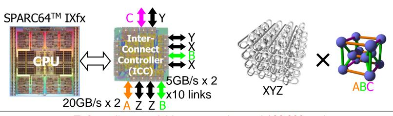
Tofu realizes scalable systems beyond 100,000 nodes With low power consumption, low latency, and high BW
