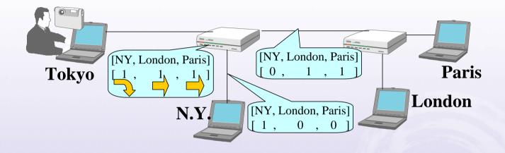
Look-up the next-hop for each address using a unicast routing table.
