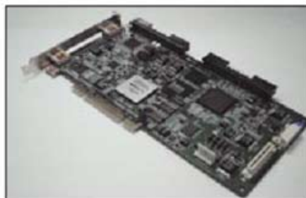
Photo 2 MB86H52 Evaluation Board
