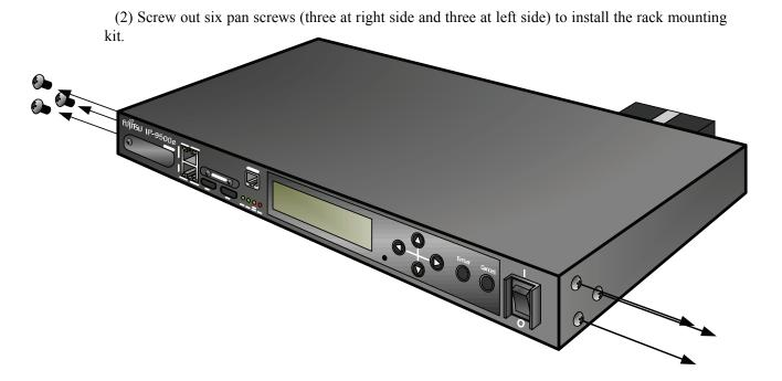
(3) Install the rack mounting kit on 19" rack using six same screws.
