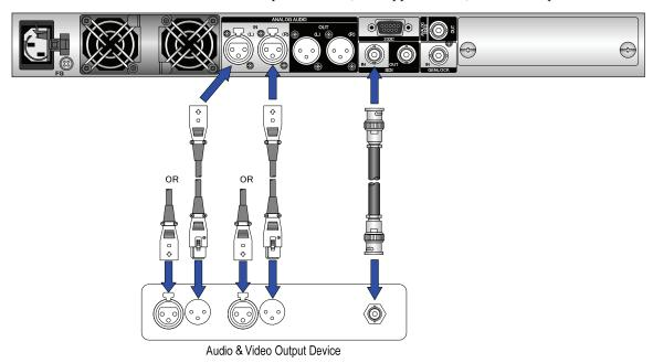
Figure Audio and video output device connections
