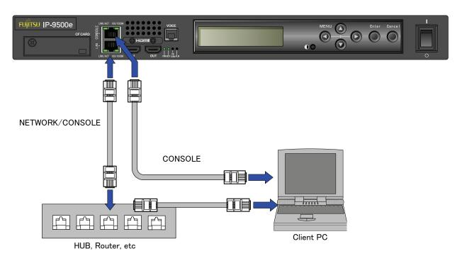
Figure Connection to a network
