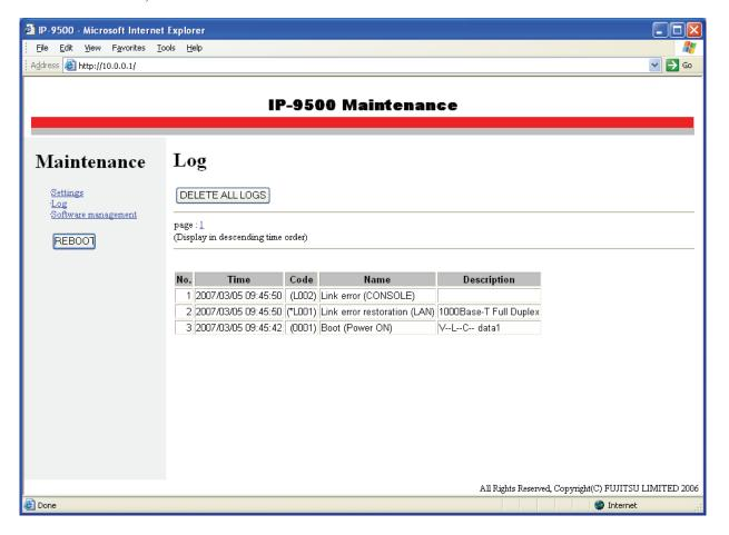
For details of the alarm log information, see the alarm code list on the next page. Note that messages may be changed after installation of each type of software. For details, see IP-9500e Software User's Guide.
