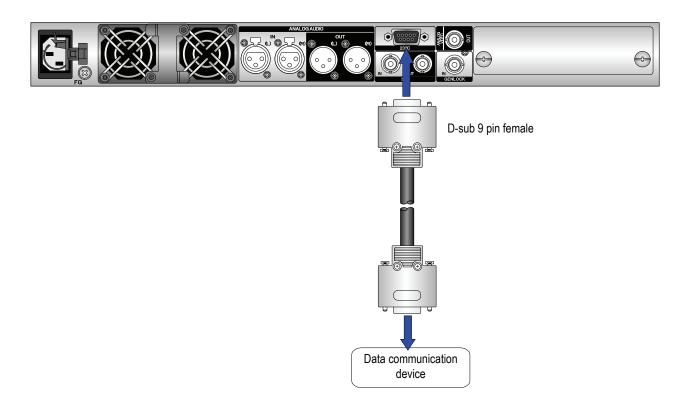
Figure Connection to RS-232C input/output device
