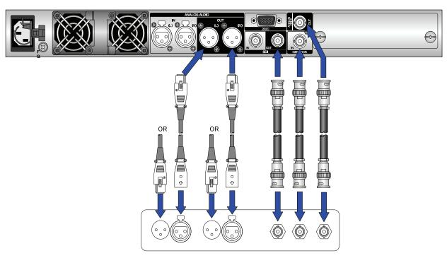
Figure Audio and video input device connections
