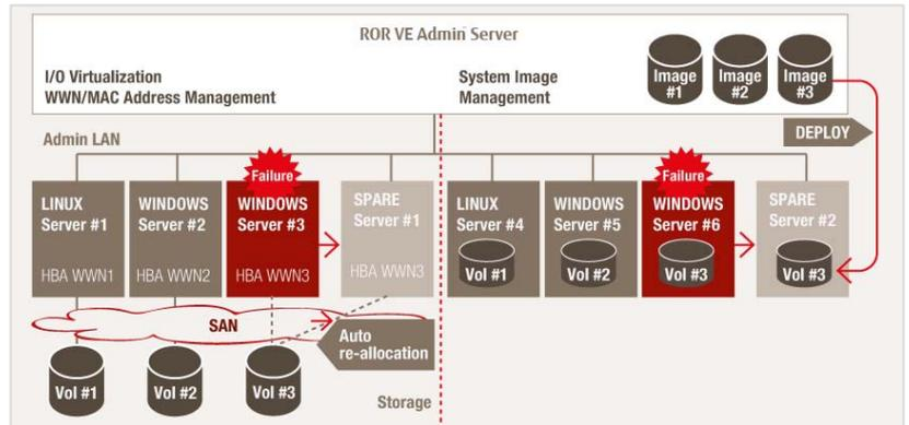
Fig 17: Server switchover in a SAN and local boot environment
