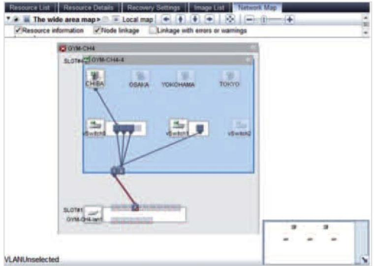
Fig 6: Integrated network map – helps server administrators to verify the network configuration
