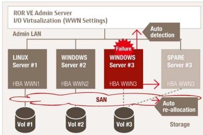
Fig 12: Automatic server failover including auto detection of server failure and auto re-allocation of storage volume
