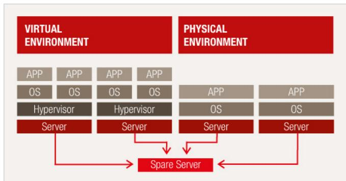
Fig 13: Sharing spare servers in mixed virtual and physical environments
