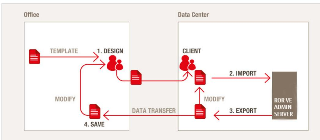
Fig 5: Setup and modification process of a ROR VE configuration
