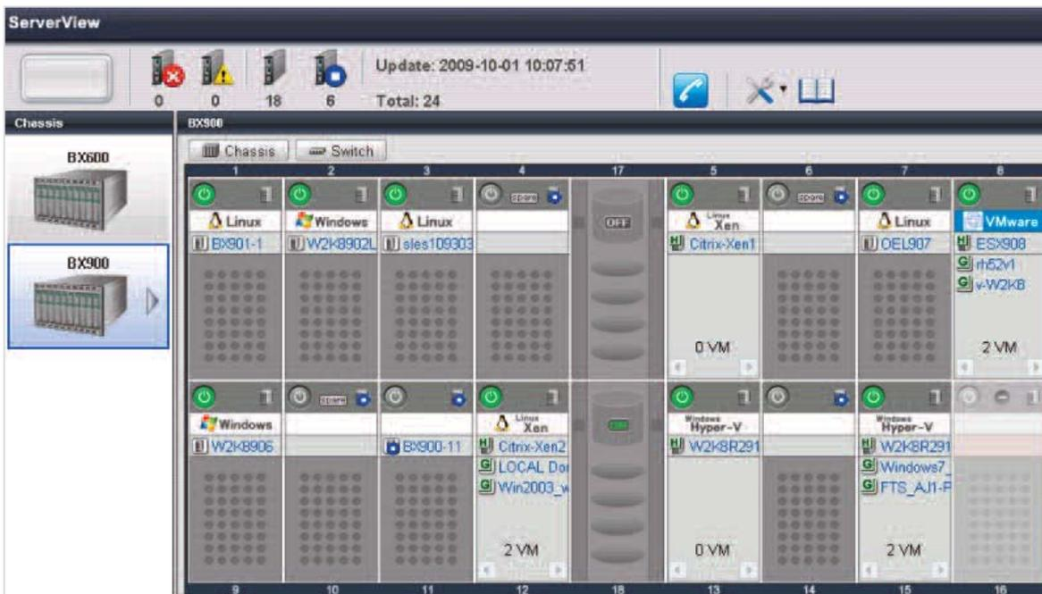
Fig 3: ROR VE BladeViewer GUI - optimized for easy daily blade server operation
