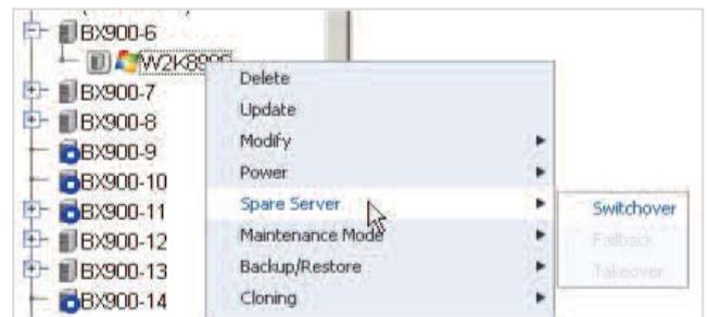
Fig 10: Initiate manual switch-over operation to a spare server
