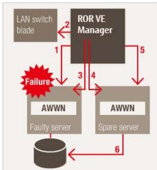
Fig 18: Server switchover using HARS
