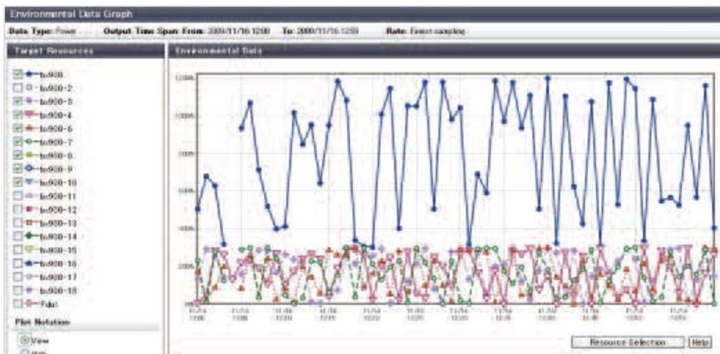
Fig 7: Tracking of power consumption trends in a PRIMERGY BX900 blade server environment
