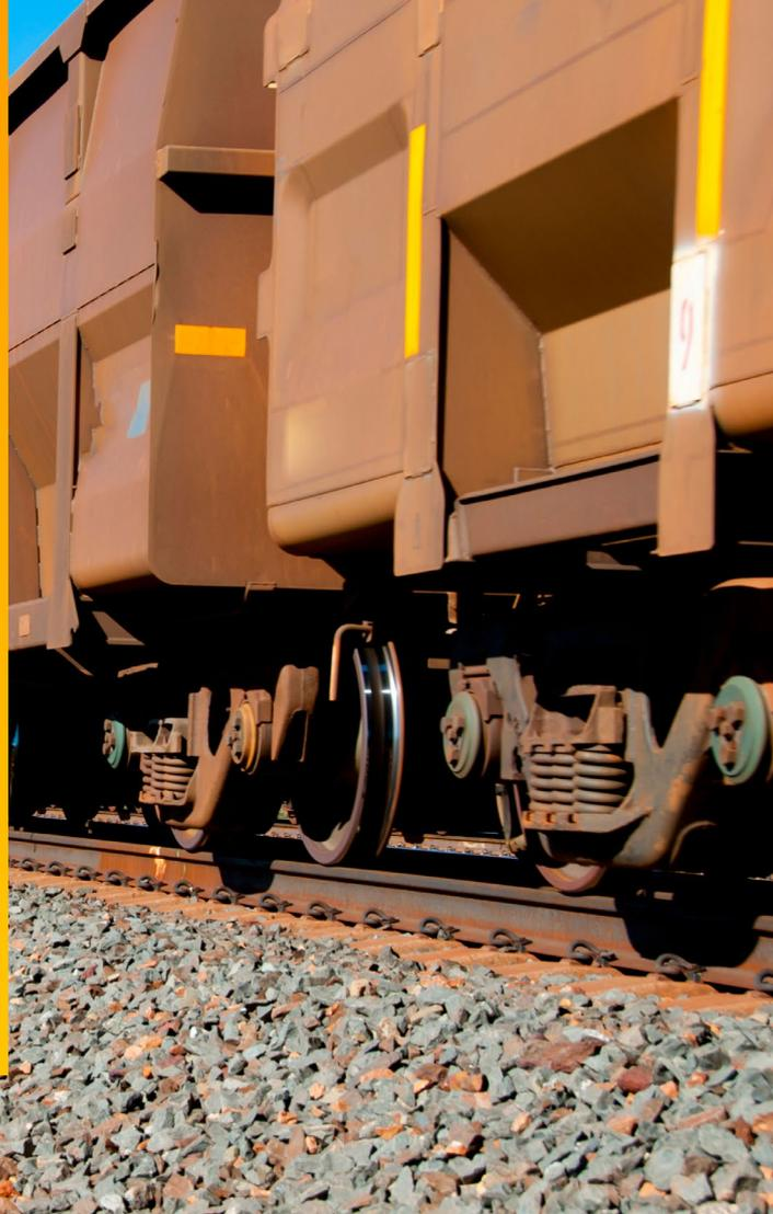
**Pacific National captures and processes high-speed images of wheelsets to determine key measurements for condition monitoring. It engaged Versor, a Fujitsu company, to develop an AI-enabled solution to calculate wagon and locomotive wheel wear characteristics and identify optimal and poorly wearing vehicle wheelsets from these measurements.**
