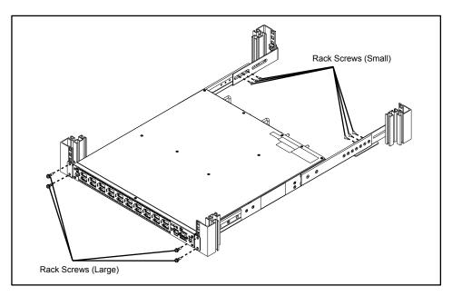
**2.** Slide the XG2000 forward, and remove it from the rack.
