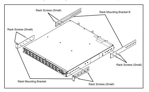
**4.** Slide the XG2000 into the rack and fasten it in place.
