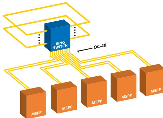
**Figure 1: Configuration of Ring Switch in a Central Office**
