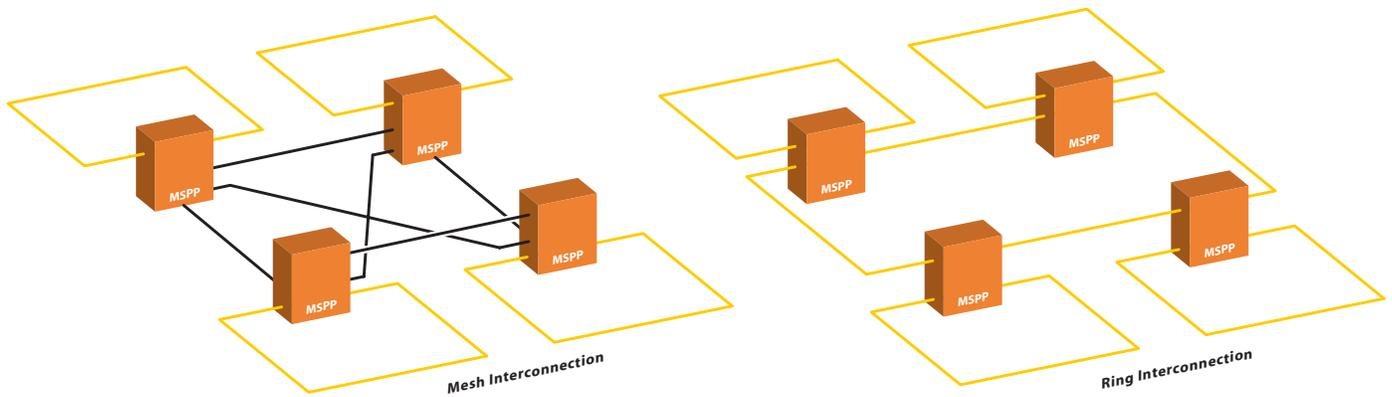
**Figure 2: Intraoffice Connections for Inter-ring Traffic using Regular MSPPs**
