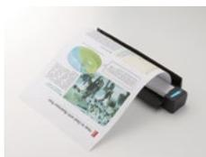
The page exits from the top of the scanner when paper path is set to U-turn.
