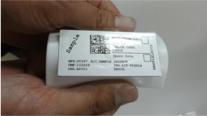
Bend down the carrier holding both longer sides to opposite direction against the carrier facing up label surface.
