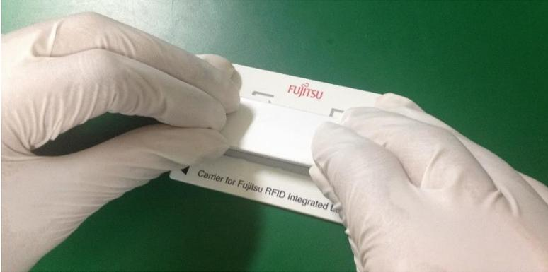
Press the RFID Label against the notch of the Reusable Carrier.
