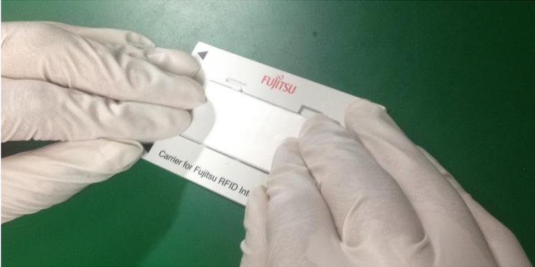
Snap the RFID Label in the cavity of the Reusable Carrier.
