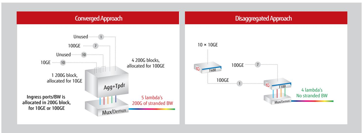
Figure 3: Less stranded bandwidth (200G versus none)
