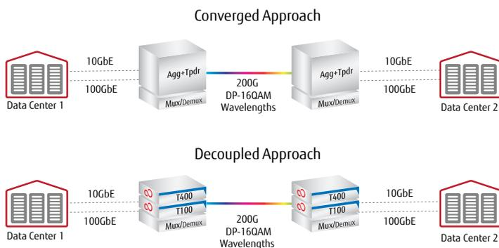
Figure 1: Comparison of Converged and Decoupled DCI Architecture
