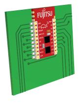
ClickBeetle evaluation boards are connecting flexible to an application PCB. ClickBeetles can be mounted by surface (SMD, only one-side assembled ClickBeetles) or by 2mm pitch through hole pin-headers (THD).
