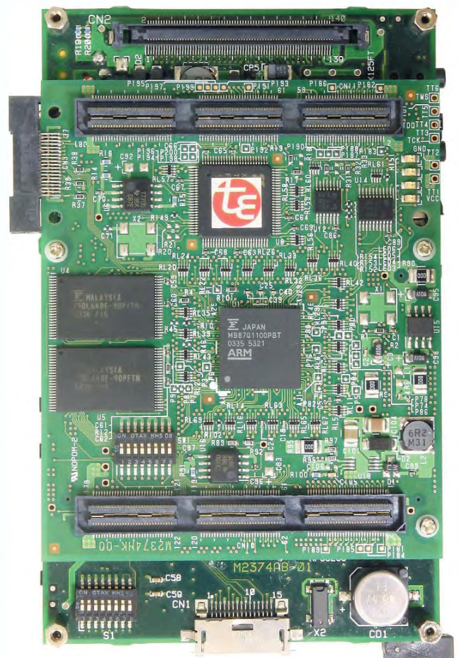
This T-Engine board (shown at actual size 120x75mm) contains Dual ARM9 platform chip MB87Q1100 and therefore offers a powerful SoC development platform.
