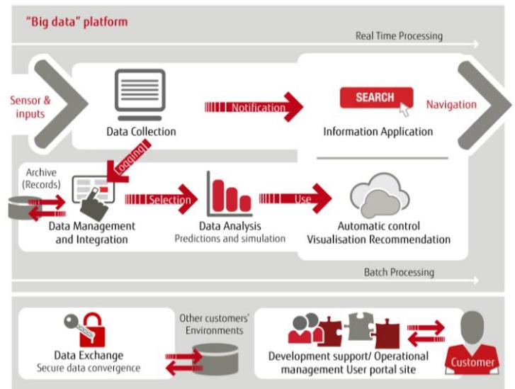
Figure 3: A functional view of a big data platform
