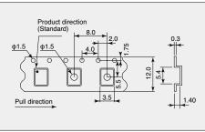
Up to 1,000 pieces per reel are boxed and shipped with the taping method shown above.
