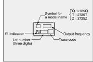
Because of space limitations, the output frequency is indicated as six digits including the decimal point. Therefore, 14.31818 MHz is indicated as 14.318.
