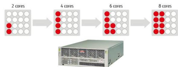
The Fujitsu M10 provides a CPU core activation function for flexible performance upgrades while also optimizing database license costs.
