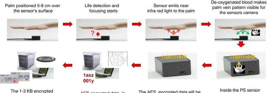
The 1-3 KB encrypted biometric template can be stored on either a PC, Server, token or smart card
