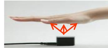
De-oxygenated blood makes palm vein pattern visible for the sensors camera
