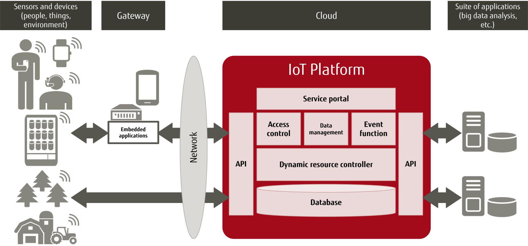
A common platform (PaaS) that enables simple and efficient usage of data from various sensors and gateways using a standard procedure.
