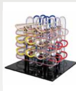
High-Dimensional Torus Interconnect Structure
