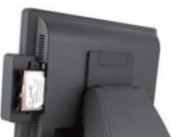
Slide in/out HDD Replacement
