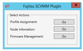
A When selecting [Profile Assignment], the ISM login console is displayed. After logging in to ISM accordingly the Node Registration screen is displayed.
