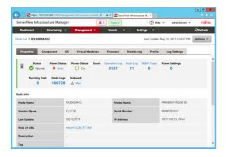
C When selecting [Firmware Management], the ISM login console is displayed. After logging in to ISM the Node information screen is displayed.
