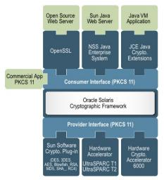
Figure 1: Oracle Solaris Cryptographic Framework is standardized and extensible—current and future cryptographic choices can easily plug in and take advantage of hardware and software capabilities.
